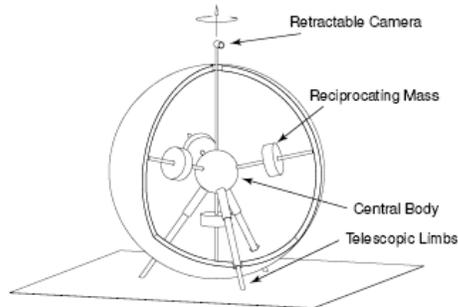
Fig. 7. The Spherobot Design
